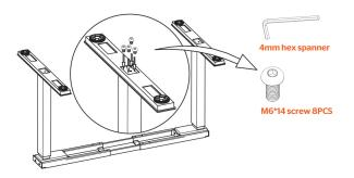
4 Attach brackets to beam using 4 of M6\*12 screws, and then fit the rubber cushion and plastic pad to the brackets and beam.
